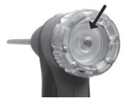
> Check the particle filter of the flue gas probe for contamination at regular intervals: check visually by looking through the window of the filter chamber. Replace the filter if there are signs of contamination.  $\succ$  Replacing the particle filter:
