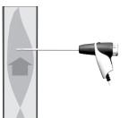
> Align the flue gas probe in the flue gas duct so that the tip is in the centre of the flow (area of the highest flue gas temperature).
