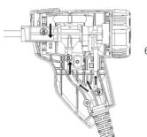
6 Connect adaptor and hose to thermocouple ((38)). Adjust lines and hoses ((99) and attach halfshells.
